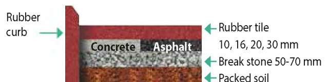
Scheme 2: Laying on a solid ground
